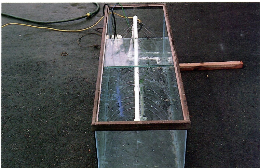
A simple rain chamber using drilled PVC and a water pump. Photo by Bob Mailloux.
